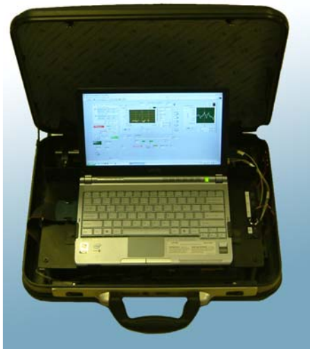
Fig 1. Photo of the compact prototype of the device intended for rapid analysis of trace quantities HF in atmosphere with the use of near-infrared diode lasers (DL) and multi-path cell.
