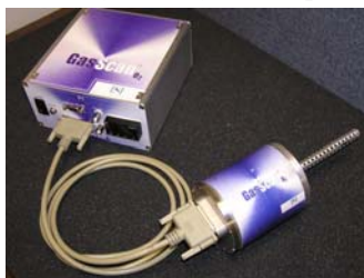
Fig.1 PSI TDLS sensor for fuel tank head space O 2 concentration, the GasScanO 2
