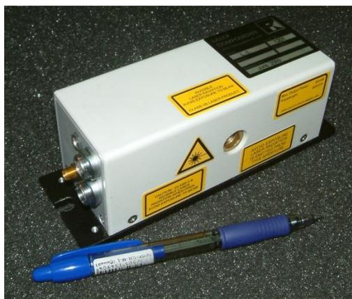
Thanks to IAEA German support program such QCL module was developed and supplied to IAEA by Laser Components (Germany) (Fig.1).
