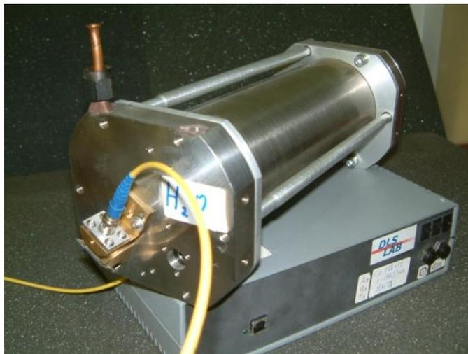
Using fiber splitters DL radiation was directed to three modules. Reference module contains cell with low pressure water vapor to stabilize DL frequency tuning. Vacuum Chernin matrix optical system ( $L = 39\text{ m}$ ) is using to measure humidity and water molecules isotopes abundance. Part of DL radiation is directed through airplane window to measure humidity variation in open atmosphere to determine turbulence parameters (see B3).
