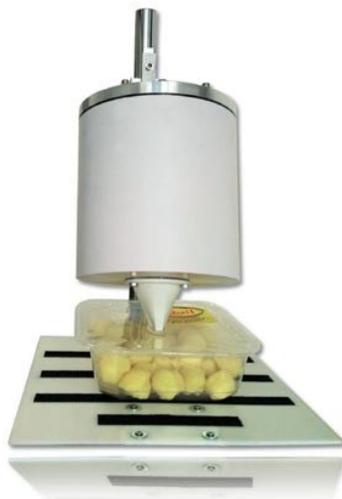
Fig.1 WMS LIDAR oxygen detection in closed Modified Atmosphere Packages. (courtesy of L Pro srl)
