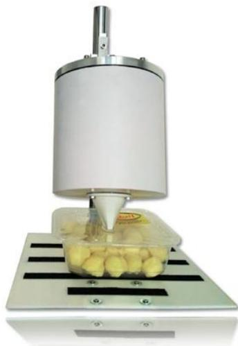
Fig.1 WMS LIDAR oxygen detection in closed Modified Atmosphere Packages. (courtesy of L Pro srl)
